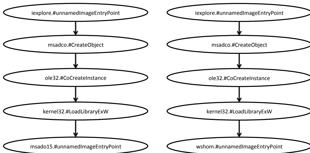
Figure 4.8: Call Sequences to Load adodb.stream and wscript.shell
