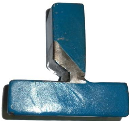
Figure A-17: Fillet Joint, Incomplete, >19mm
