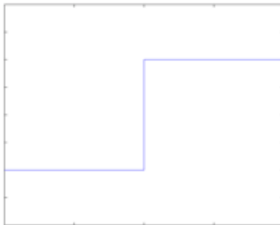
Figure 6.2: A discrete, digital signal.
