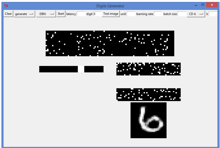
Figure 31: Image generated by the model when clamping a 6 to the label units
