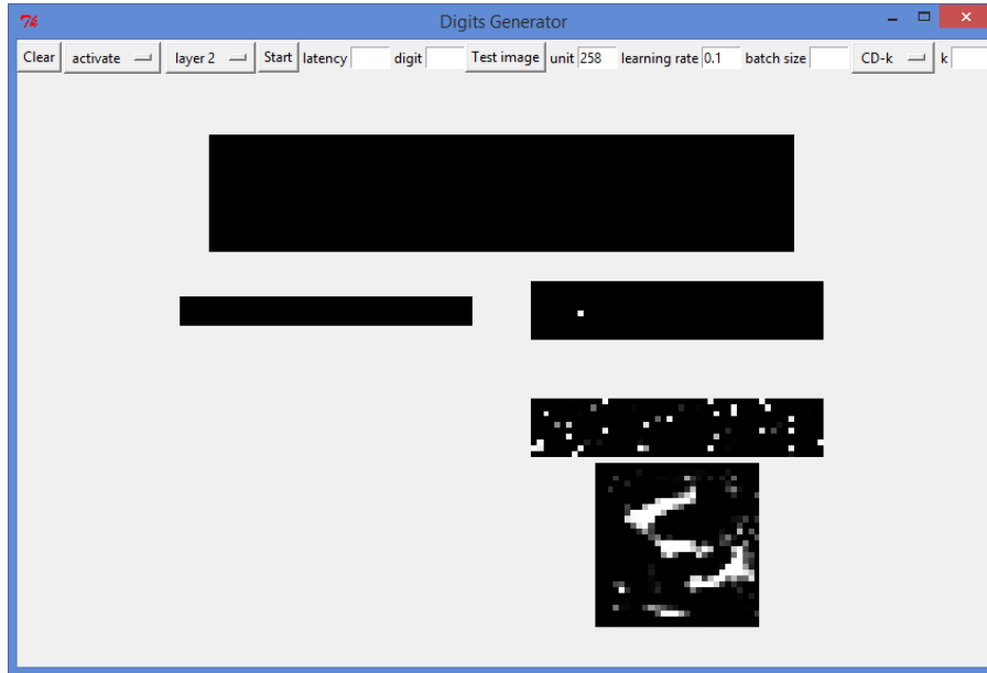
Figure 35: Input image maximizing the activation of a given unit in the layer h2. Image obtained by numerical optimization with backpropagation.
