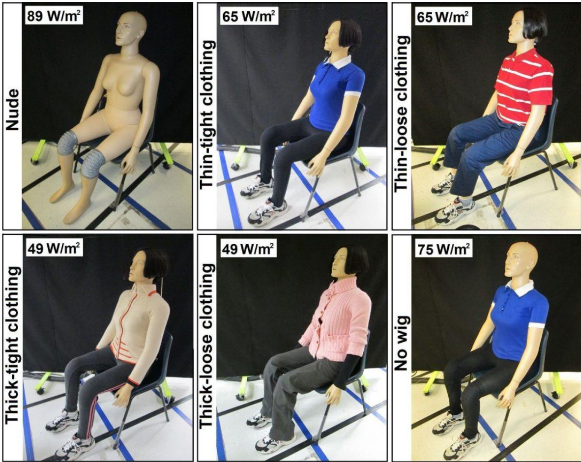
Figure 3.2 Thermal manikin with different levels of clothing insulation/design.
