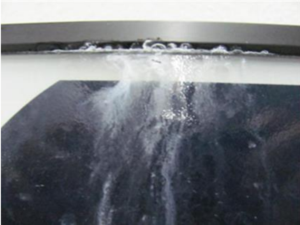
Fig. 36. Glass surface deterioration of mono-Si backcontact module after the positive bias Damp Heat 85/85 test. White “mist” on front glass and frame corrosion are also shown.
