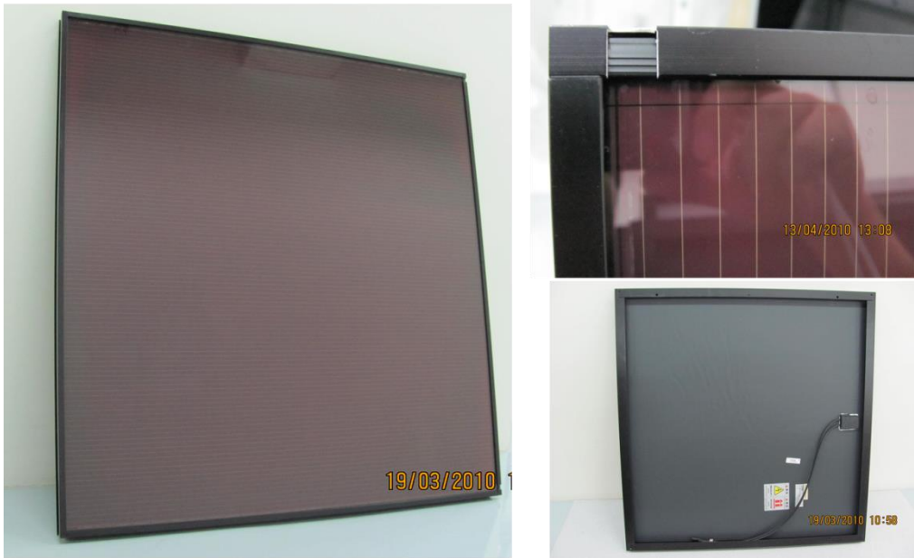
Fig. 18. Photos of a-Si PV module. Size: 990 x 960 x 40 mm. Glass-Backsheet structure with frame and thick edge sealing rubber.
