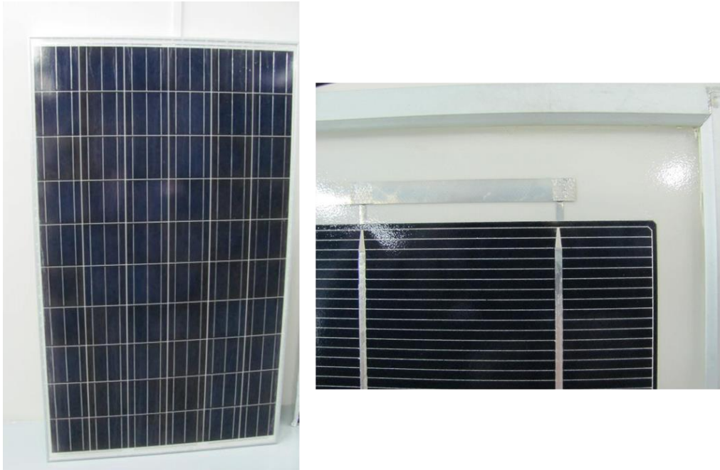
Fig. 24. Photos of multi-Si PV module. Size: 1650 x 992 x 46 mm. Glass-Backsheet structure with frame and edge sealing adhesive.
