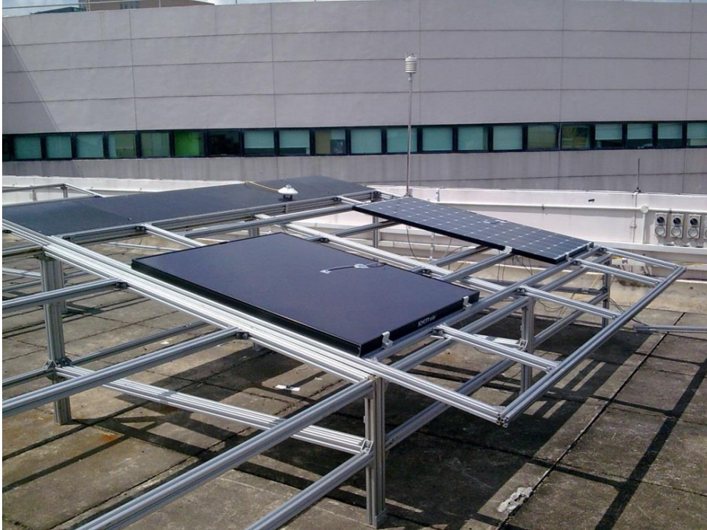
Fig. 48. NOCT sg test for an amorphous Si tandem PV module and a heterojunction mono-Si/a-Si module in Singapore.
