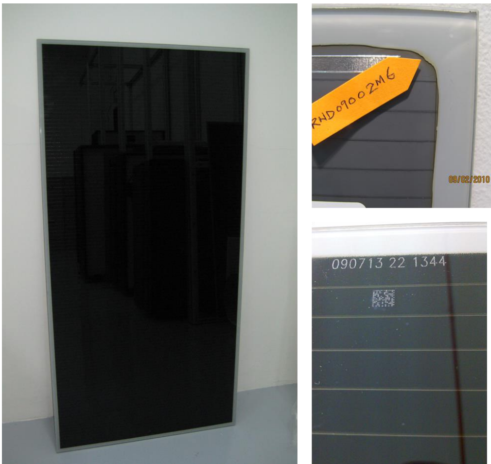
Fig. 19. Photos of CdTe PV module. Size: 1200 x 600 x 6.8 mm. Glass-Glass structure without frame but with edge sealant.
