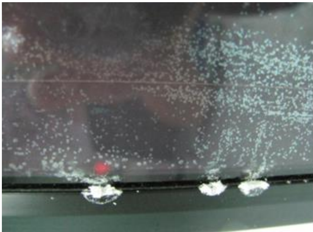
Fig. 35. “Dot-like” delamination at thin-film layer under the front glass of a-Si/a-Si tandem module after the positive-bias Damp Heat 85/85 test; Frame corrosion is also shown.
