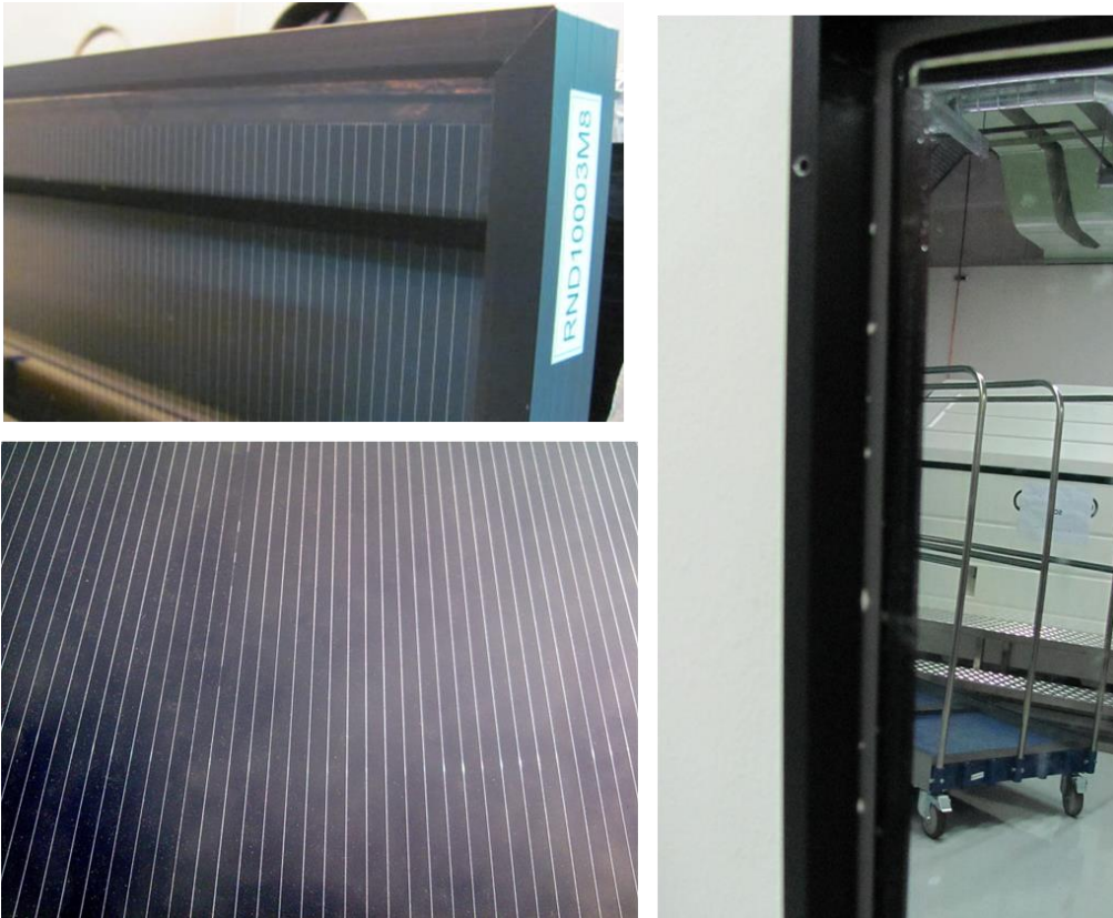
Fig. 22. Photos of CIGS PV module. Size: 1235 x 641 x 35 mm. Glass-Glass structure with frame and edge sealant.
