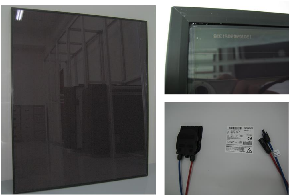
Fig. 20. Photos of a-Si/a-Si tandem PV module. Size: 1308 x 1108 x 50 mm. Glass-Backsheet structure with frame and edge sealing tape.
