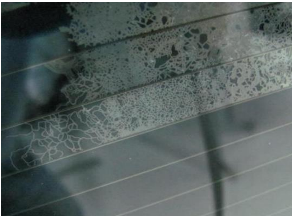
Fig. 33. “Hair-like” delamination at thin-film layer under the front glass of CdTe module after the negative bias Damp Heat 85/85 test.
