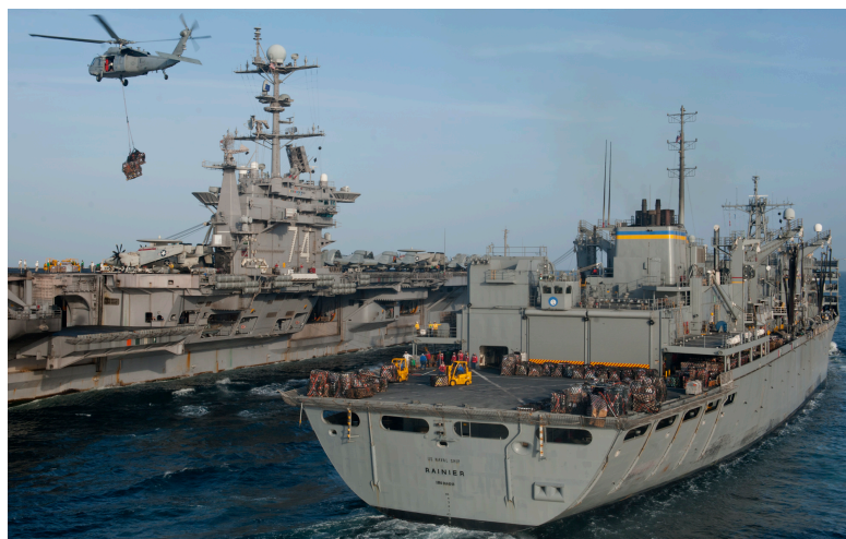
Figure 1.1: Vertical replenishment by U.S. Navy (Use of released U.S. Navy imagery does not constitute product or organizational endorsement of any kind by the U.S. Navy.)
