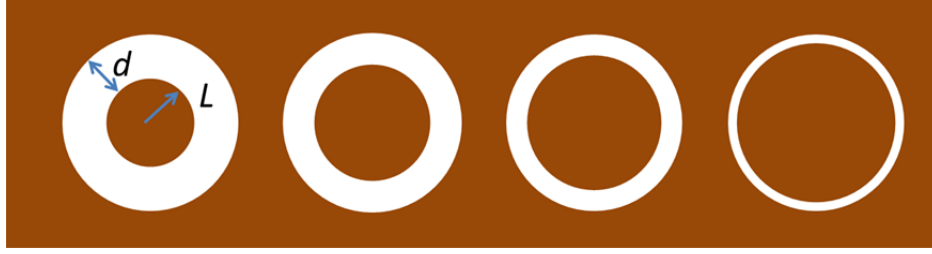
Figure 2.10 Circular transmission line method test structure with various spacing d and same radius L . The brown areas indicated metallic regions.
