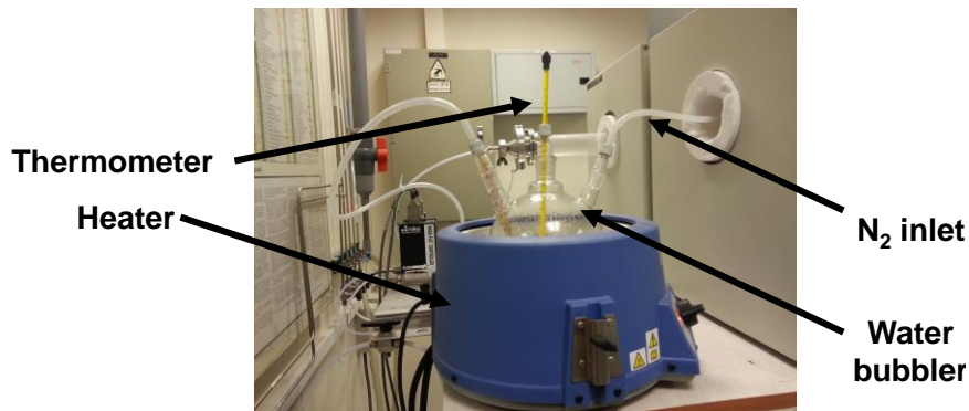
Figure 6.3: The wet oxidation setup showing the furnace, the water bubbler, and the N 2 inlet
