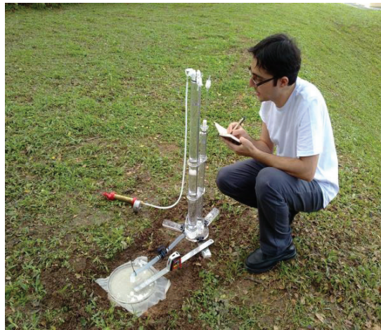
Figure 3.5: Measuring of tension infiltrometer data
