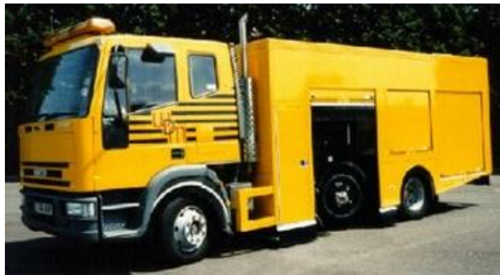
Figure 2.10: Sideway-force coefficient routine investigation machine (SCRIM)
