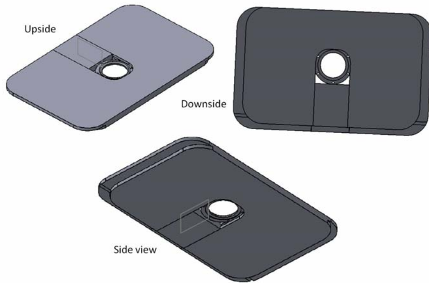
Figure 3-4. Different views of mice imaging window design. This design is revised based on the second generation rat imaging window design, but it is in a much smaller size. It could be stabilized to the microscope's sample plate like histology slides. This feature makes it able to adapt to different microscope models.
