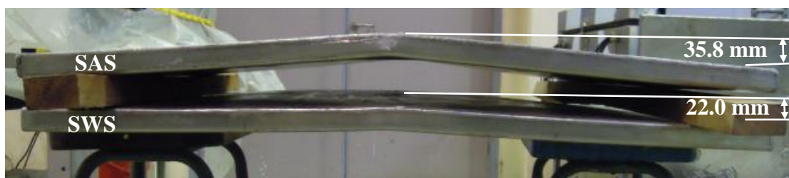
Fig. 5.9 Permanent deformation of SAS and SWS after 2 nd test
