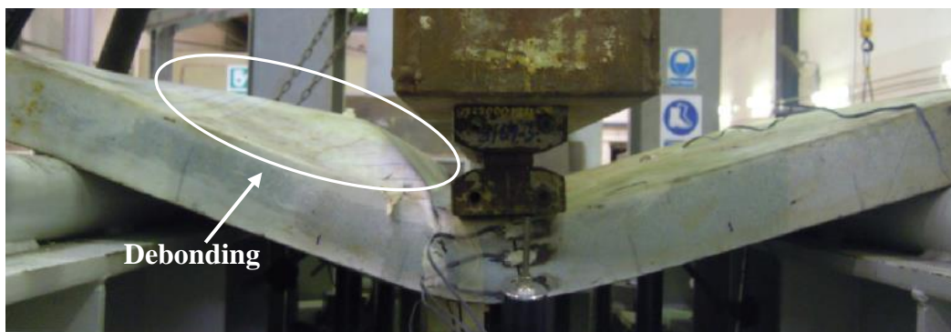
Fig. 4.21 Flexure failure of SCS75 panel under line load
