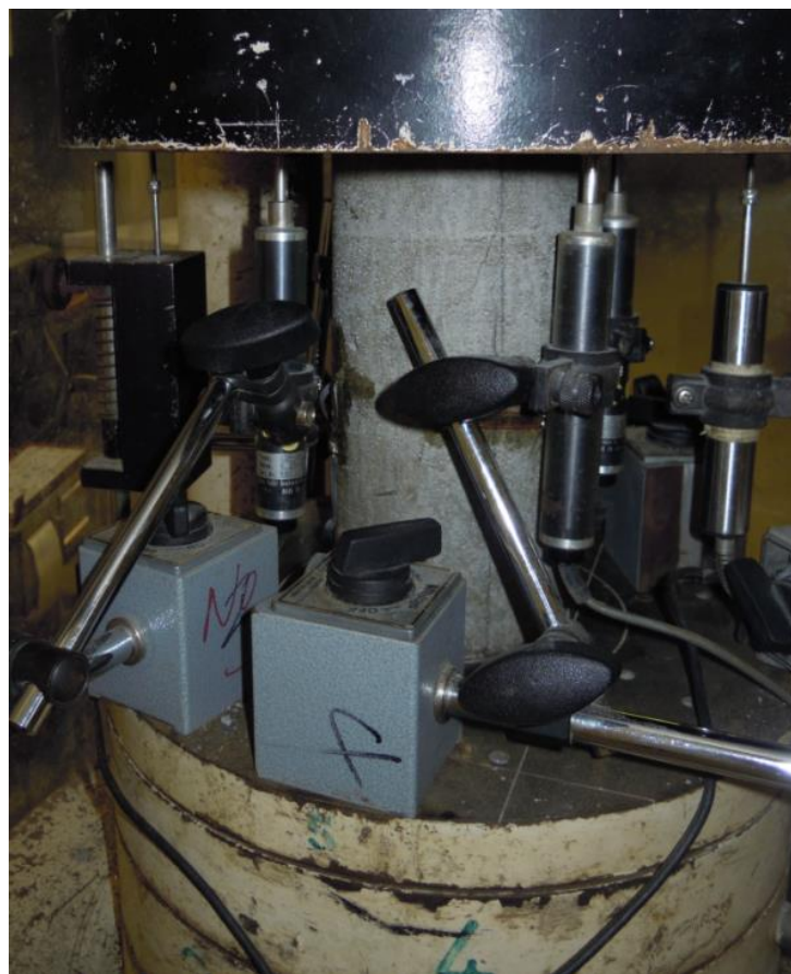
Fig. 4.4 Uniaxial compression test setup
