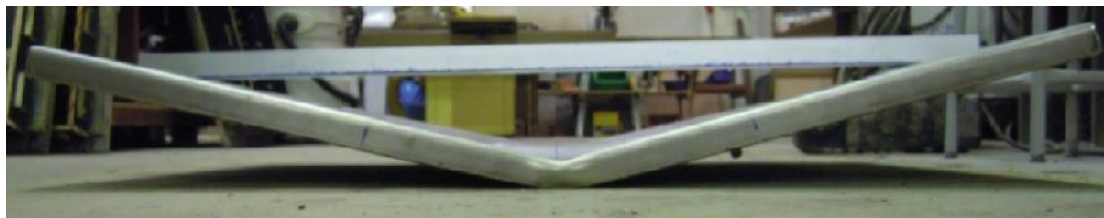
Fig. 4.15 Flexural failure of SAS tank
