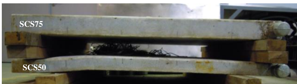
Fig. 5.11 Deformed shape of SCS50 and SCS75 panels after impact
