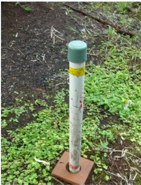
Fig. 4.1: Monitoring pole for water table depth and peat subsidence measurements
