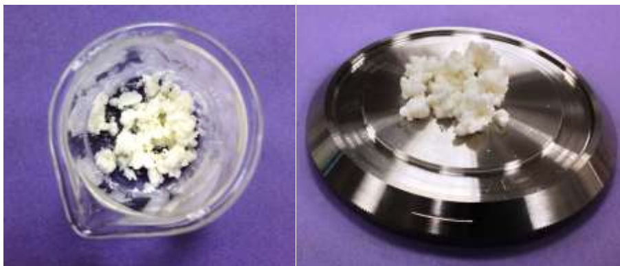
Figure 6.3 Physical appearance of CS suspended in water for concentration just above the maximum packing fraction ( \phi_m )
