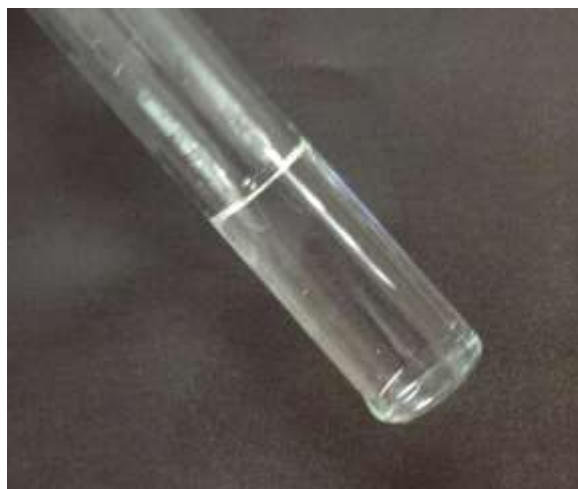
Figure 1.4 Clear gel formed in 20% Pluronic F127 at 40°C
