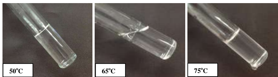
Figure 5.7 Images of tilted glass tubes with the mixture 12.5% F127 + 12.5% L64 at different temperatures; the sample appearance did not change after one week
