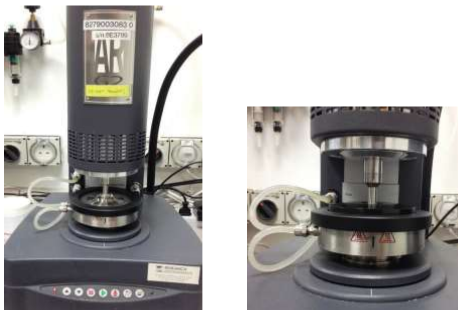
Figure 2.4 Image of rheometer AR G2 with cone and plate geometry (left) and with the solvent trap (right)
