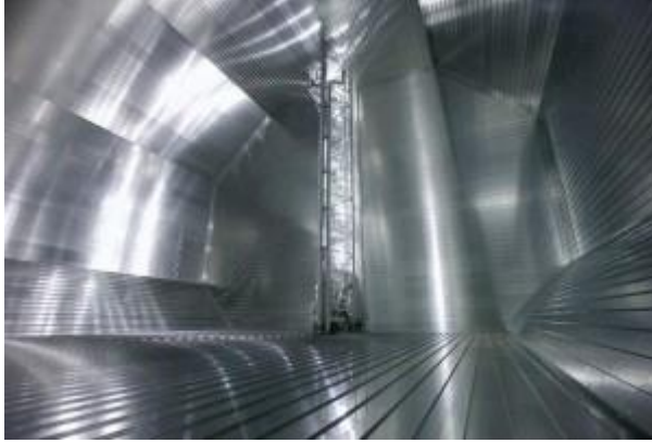
Figure 1.5: Interior of a membrane type tank in an LNG carrier (Source: GTT)
