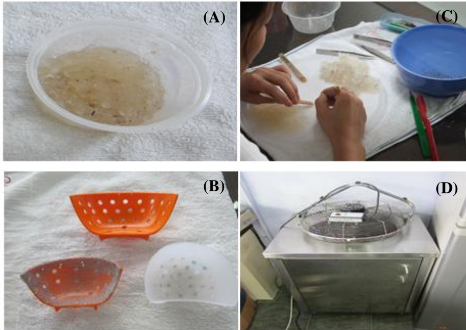
Figure 6 Graphical display of the processing method for EBN. (A) soaking of EBN in water (B) manual removal of the impurities from EBN (C) the moulds which shape the EBN into a half bowl shape. (D) the oven for the drying of EBN.
