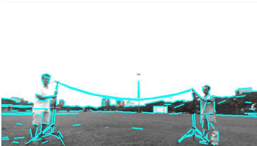
Figure 3.26: Line segment detector applied to powerline image.
