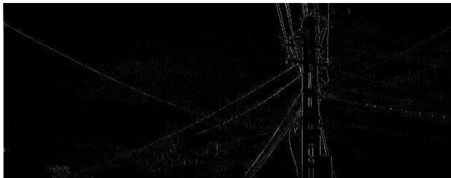
Figure 3.24: Sobel kernel filtering in \delta y .
