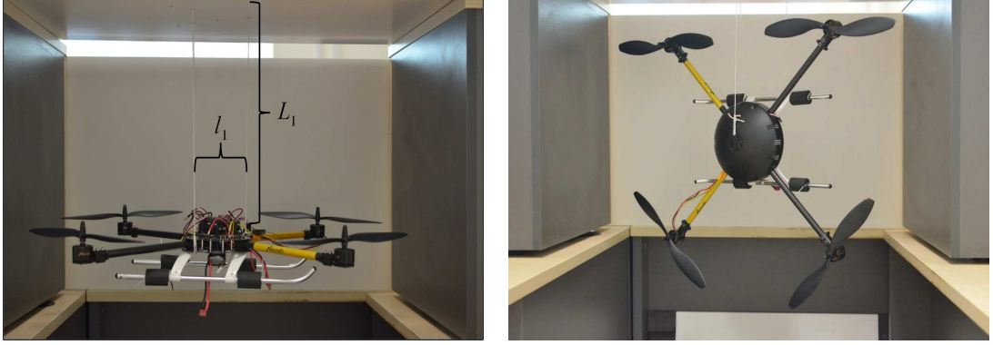
Figure 2.13: Left: J_{zz} measurement, Right : J_{xx}, J_{yy} measurement.
