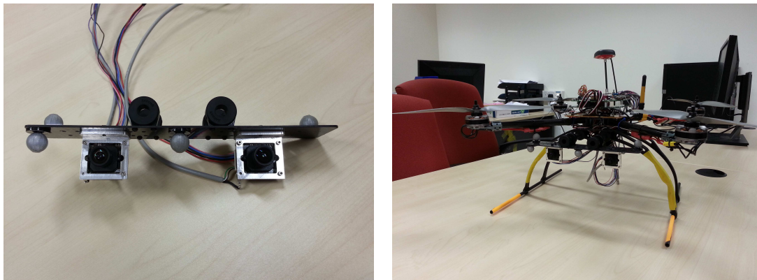
Figure 3.2: Left: Customized stereo camera, Right: Stereo camera mounted on Quadrotor.
