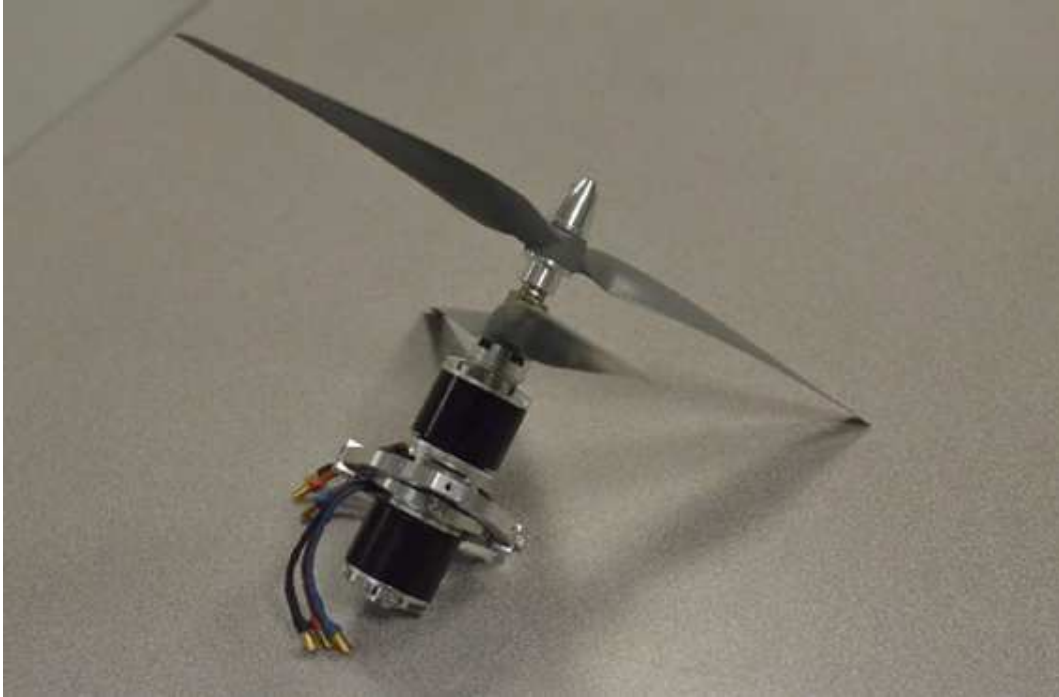
Figure 2.36: The self-customized contra-rotating motor.
