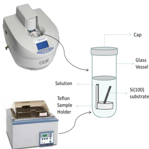
Figure 2.7 The setup of microwave heater (CEM Discover), water bath heater (PolyScience) and glass bottle.
