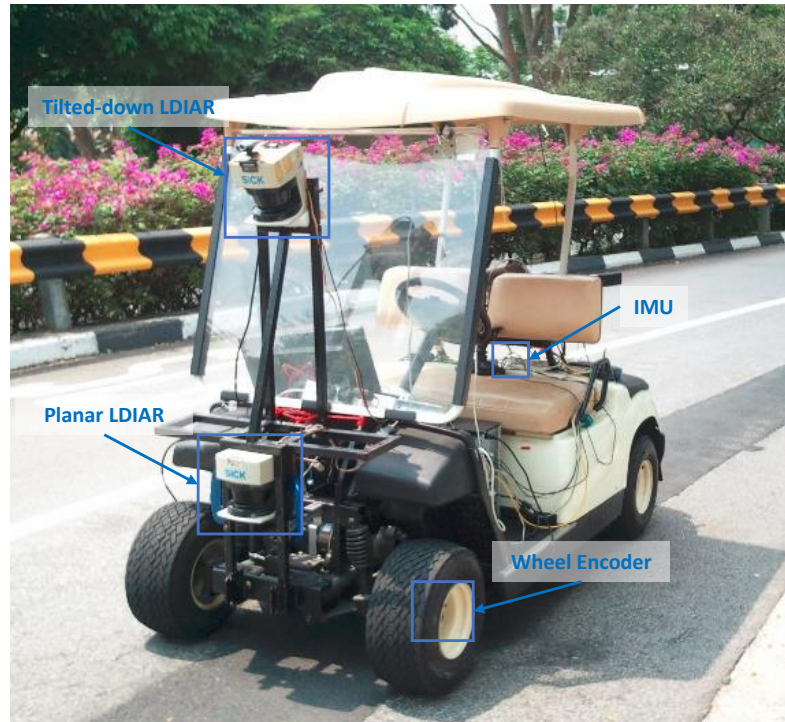
Figure 3.9: Yamaha G22E golf cart mounted with various sensors
