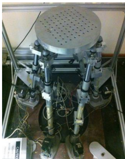
Figure 3.20 The components and final construction of the SP
