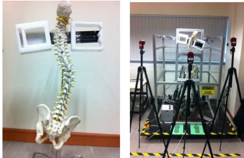
Figure 5.2 Mechanical frame and anthropometric marking position on the physical spinal model
