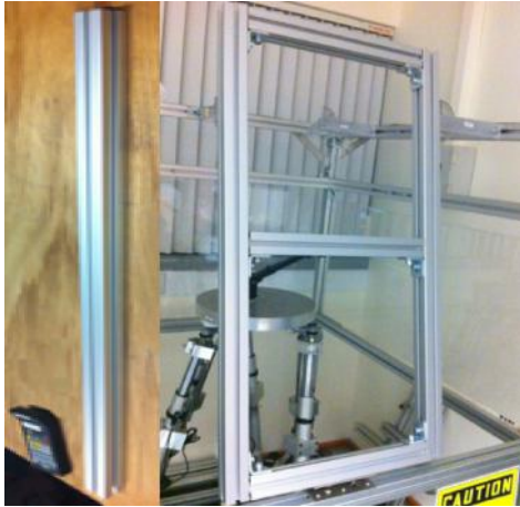
Figure 3.18 Aluminum bar and the assemble of the mechanical moveable plate Figure 3.19 Sign of the foot step
