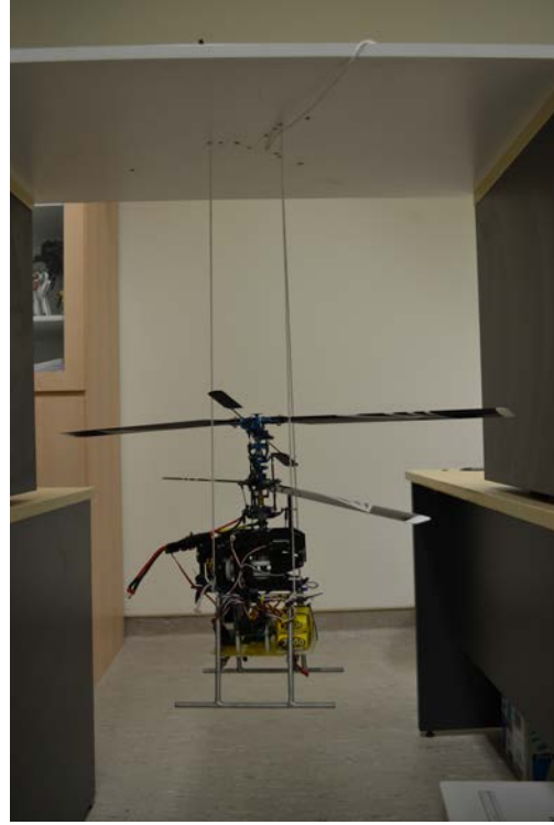
(b) Measurement setup of trifilar pendulum.
