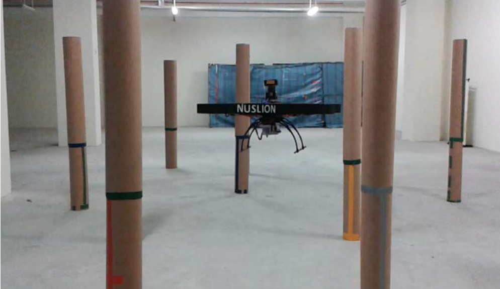
Figure 4.16: The indoor test scenario for verifying scan matching.
