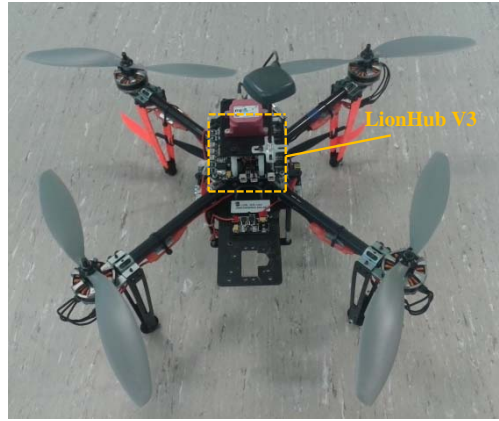
(b) LionHub V3 on quadrotor for IMAV2014
