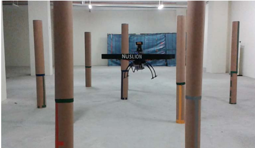
Figure 6.7: Indoor test scenario for GraphSLAM verification.
