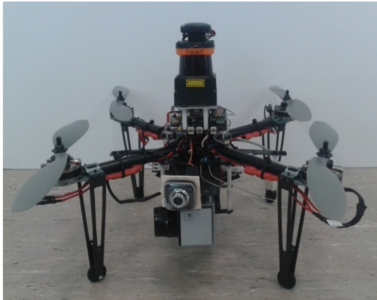
Figure 2.10: NUS quadrotor platform with two onboard laser range finders.
