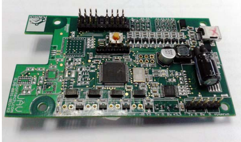
Figure 2.21: One-board configuration of servo control board: UAV100.
