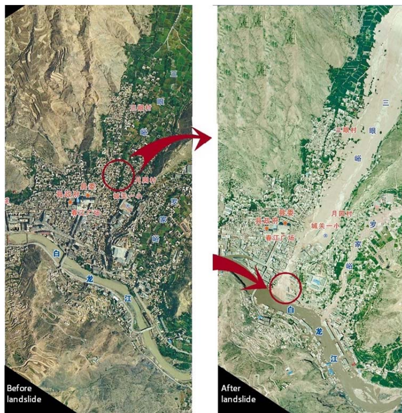
Figure 3.6 Pre- and post-landslide aerial-image comparison on the landslide occurred on August 8, 2010 in the upper reach of the Jialing River; images were provided by the National Administration of Surveying, Mapping and Geoinformation of China. The arrow in the left panel indicates the residential area, which has destroyed and
