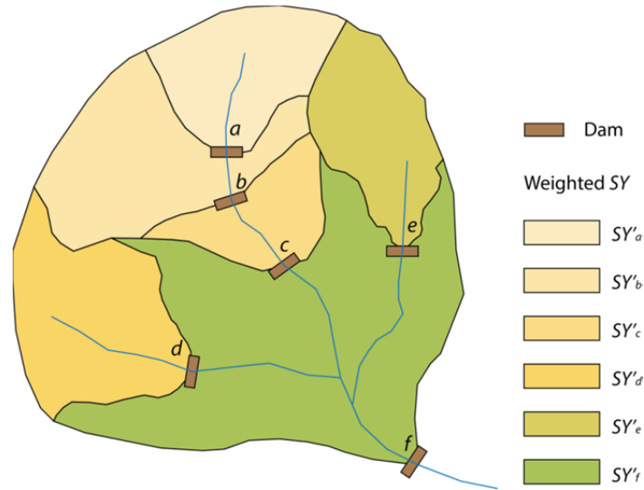
Figure 5.2 Protocol for predicting reservoir sedimentation in a multi-reservoir system. Reservoir f is the farthest downstream; reservoirs a , d , and e are immediately upstream of f and they are direct sediment-contributing reservoirs to reservoir f . Reservoirs c , d , e are representative reservoirs that have no upstream reservoirs. SY' is weighted sediment yield for each reservoir, for example, sediment yield at reservoir f is the sediment yield in SY'_f plus the sediment released from its immediately upstream reservoirs a , d and e .
