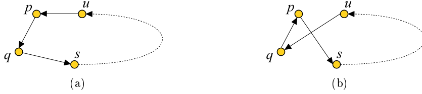
Figure 8.3: Twisting edge \overrightarrow{pq} of the polygon in (a) leads to the polygon in (b).
