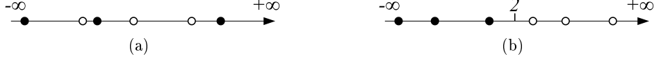
Figure 9.4: (a) A time line that is not well-separated and (b) a well-separated time line at t = 2 . Positive nodes are in black while negative ones are in white.
