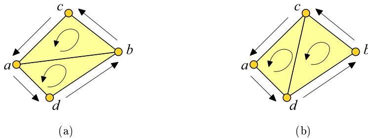
Figure 8.5: Flipping \overline{ab} on a coherently oriented triangulation.
