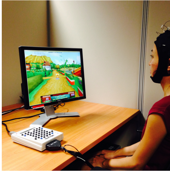
Figure 5.6: Experimental setup to collect EEG data during NF training sessions. Subjects should modulate their brain signals to move the avatar on the screen. The BCI score which is shown on the bottom left corner of the screen is the speed of the avatar.
