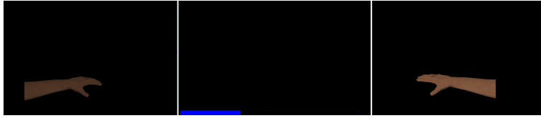
Figure 5.3: A visual cue in MI-BCI experiment. The left (right) hand instructs subject to perform left (right) hand MI. The horizontal blue bar showed the preparation time before providing a cue.
