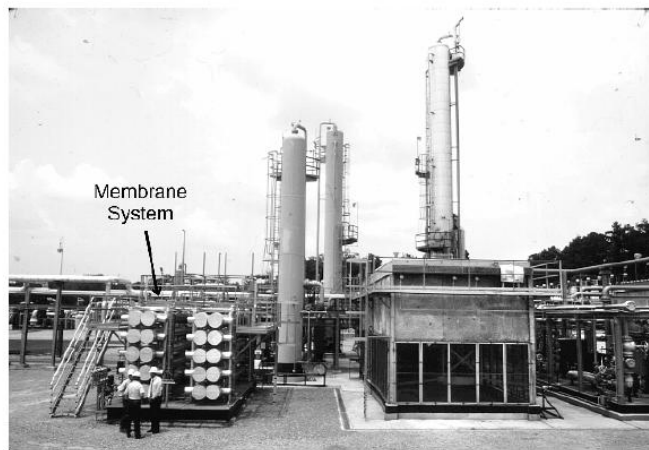
Figure 1.3 Size comparisons of membrane and amine system [9]
