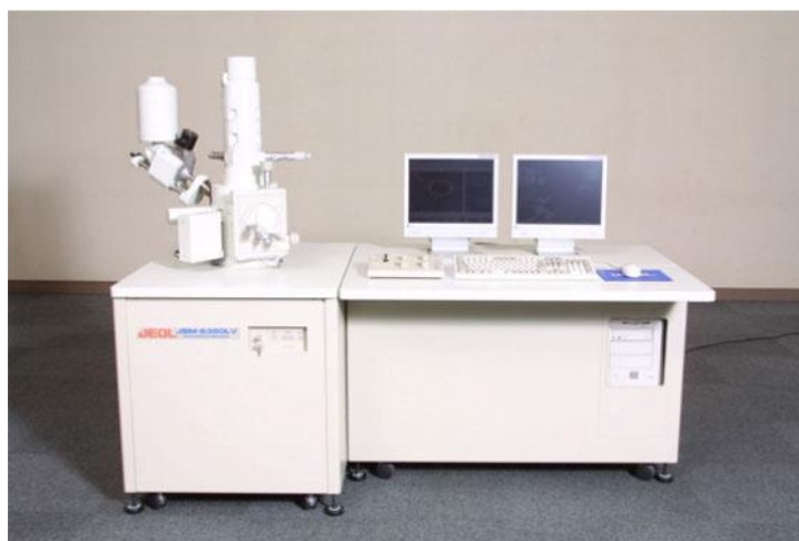
Figure 3.11 Scanning electron microscope (JEOL JSM-6360LA)
