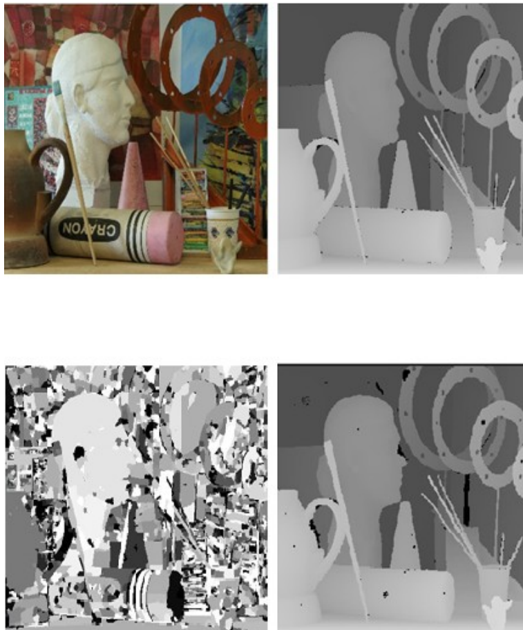
Figure 4.12 Experimental results of Arts. (a) reference image; (b) disparity map provided in Middlebury database; (c) initial disparity map; (d) disparity map obtained by the proposed algorithm.
