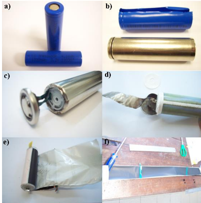
Figure 3.2 (a) 18650 cell. (b) After stripping off the heat shrink wrapping. (c) Positive terminal. (d) Negative terminal. (e). Unwinding the current collectors. (f). Tab and coated electrode.
