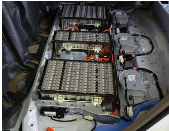
Figure 2.5 Toyota Highlander hybrid battery pack.
