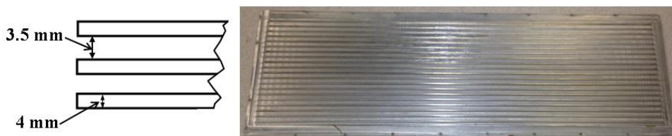
Figure 9.2 Straight channel fin.
