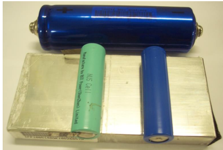
Figure 6.1 Various types of heat shrink wrapping for Li-ion battery.
