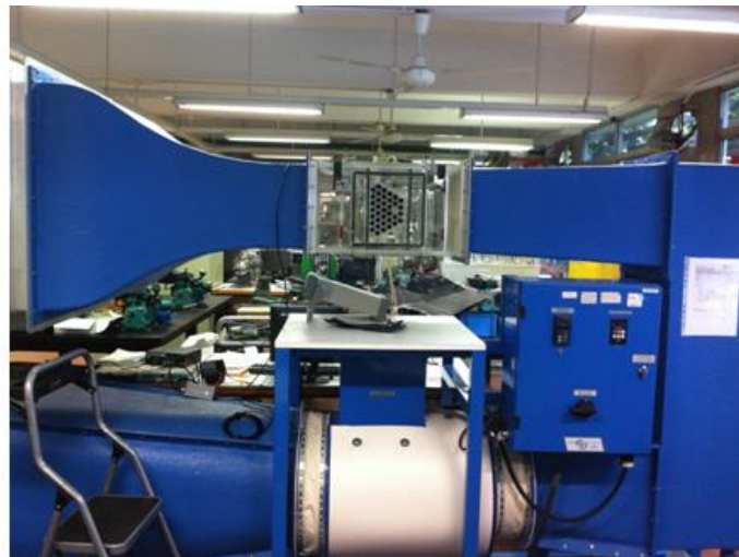
Figure 8.14 Experimental setup on the wind tunnel.
