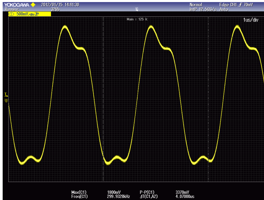
Figure 6.18: Distorted output waveform from one power amplifier
