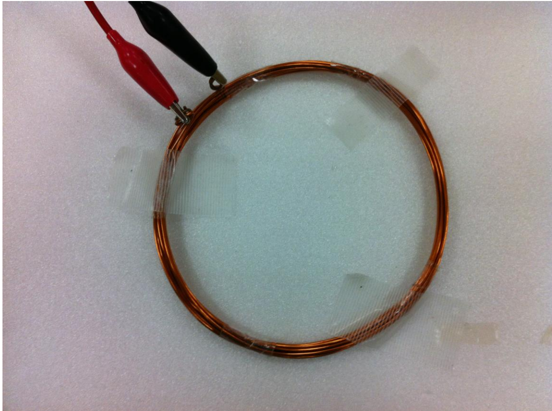
Figure 6.20: Power transmitting coil for 2-step power amplifier
