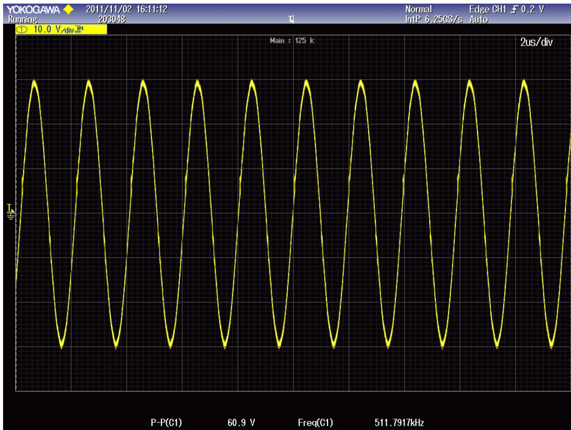
Figure 6.12: Example output waveform of power transmitter: f = 511\text{kHz}
