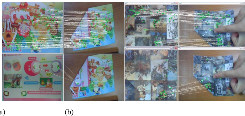
Figure 4.7: Test of Different Paper Tracking using SURF: (a) postcard, (b) newspaper
