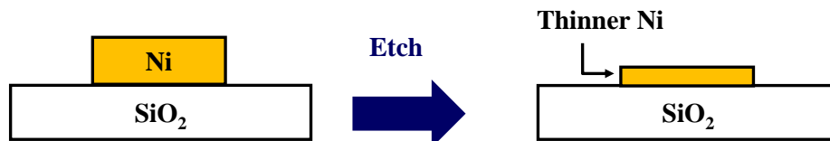
Fig. 3.2. Schematic of the samples used for determining the etch rates of Ni-InGaAs and Ni; (a) Unpatterned or blanket sample comprising of Ni-InGaAs formed on \text{In}_{0.53}\text{Ga}_{0.47}\text{As}/\text{InP} substrate, (b) blanket sample comprising of Ni deposited on silicon dioxide ( \text{SiO}_2 ) on a Si substrate, and (c) patterned Ni film formed on \text{SiO}_2 on Si.
