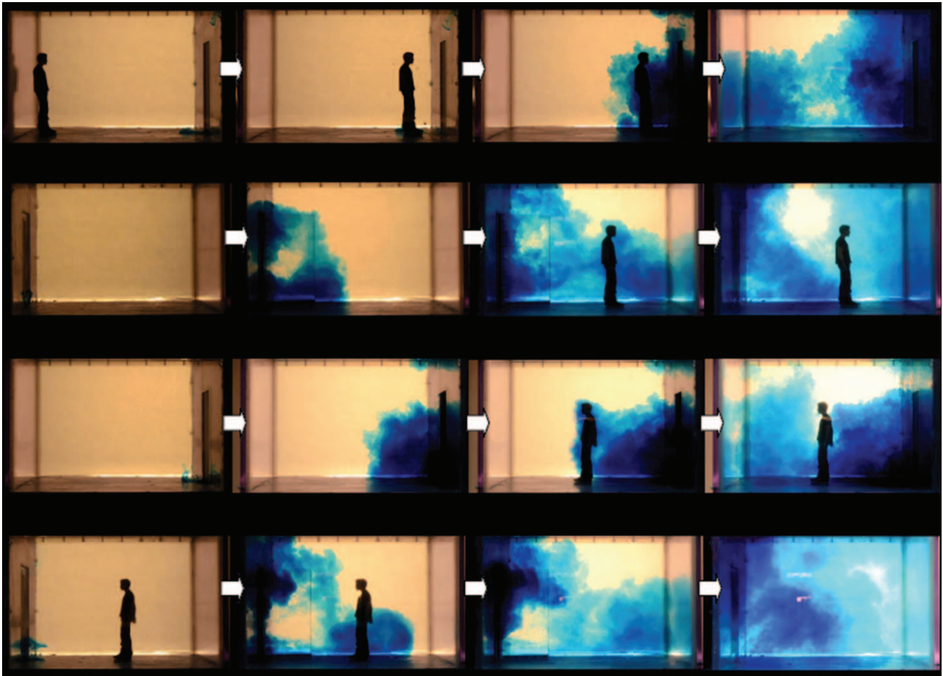
Figure 5. Single-hinged door snapshots (sideviews only; left-to-right). The series of 4 snapshots with each door-opening, manikin movement scenario were taken with respect to the following events, rather than at specific times: food dye movement due to door-opening motions alone then with any initial manikin movement – manikin interaction and any entrainment food dye – final food dye movements once the manikin had come to rest at its destination position. All movement parameters are shown in Table 2 for these single-hinged door ‘fast’ scenarios. A. Manikin moving into the isolation room (seen from outside, V_1 = 0.79 in water (1.22 in air) m/s, angular velocity = 184.68 in water (28.63 in air) deg/s). B. Manikin moving into the isolation room (seen from inside), V_2 = 0.75 in water (1.17 in air) m/s, angular velocity = 184.68 in water (28.63 in air) deg/s. C. Manikin moving out of the isolation room (seen from outside), V = 0.77 in water (1.19 in air) m/s; angular velocity = 184.68 in water (28.63 in air) deg/s. D. Manikin moving out of the isolation room (seen from inside), V = 0.77 in water (1.19 in air) m/s; angular velocity = 184.68 in water (28.63 in air) deg/s.
