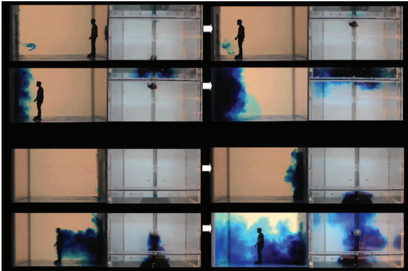
Figure 4. Double-sliding door snapshots (side and top views; left-to-right, top-to-bottom). The series of 4 snapshots with each door-opening, manikin movement scenario were taken with respect to the following events, rather than at specific times: food dye movement due to door-opening motions alone then with any initial manikin movement – manikin interaction and any entrainment food dye – final food dye movements once the manikin had come to rest at its destination position. All movement parameters are shown in Table 1 for these double-sliding door scenarios. Note that with the sliding doors, the scenarios where the manikin enters or leaves the isolation room are effectively symmetrical (unlike with the hinged-door scenarios). A. Manikin moving into/out of the isolation room (seen from outside/inside, respectively), V = 0.79 in water (1.22 in air) m/s, door-opening gap velocity = 0.42 in water (0.64 in air) m/s. B. Manikin moving out of/into the isolation room (seen from outside/inside, respectively), V = 0.79 in water (1.22 in air) m/s, door-opening gap velocity = 0.42 in water (0.64 in air) m/s. doi:10.1371/journal.pone.0066663.g004
