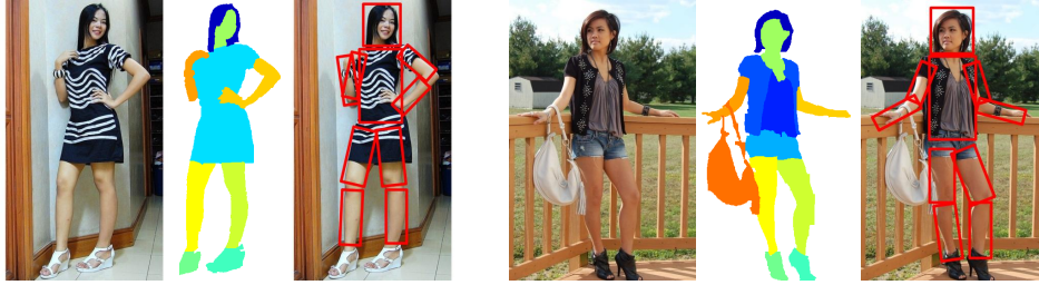
Figure 4.2: Human decomposition based on different basic elements. The original image, Parselet based decomposition and joint based decomposition are shown sequentially.
