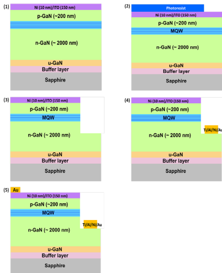
Figure 6.7 Schematic diagrams of the fabrication steps of GaN LED.
