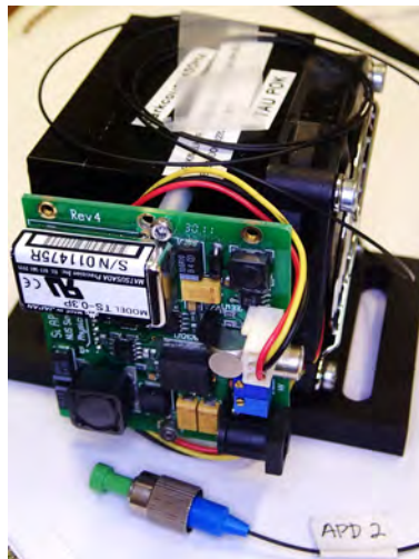
Figure 4.2: A fiber pigtailed APD module, showing the electronics needed to provide a high bias voltage to the APD, quench the APD, and to provide a NIM output signal for each photon detection event.
