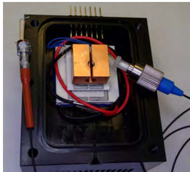
Figure 4.1: A fiber pigtailed APD module under assembly. The diode is seen to the left, and a black multimode fiber has been glued in place illuminating the active surface of the diode. The APD sits in a copper housing atop a three stage Peltier element used to cool the diode. To prevent condensation the whole structure is mounted in a black air tight aluminum housing.
