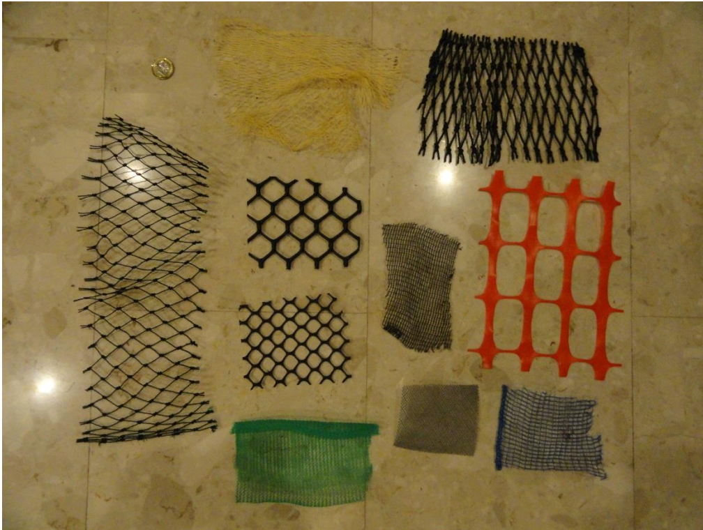
Fig. B.5. Proposed mesh materials for anti-predator cages. In situ biofouling tests were performed.
