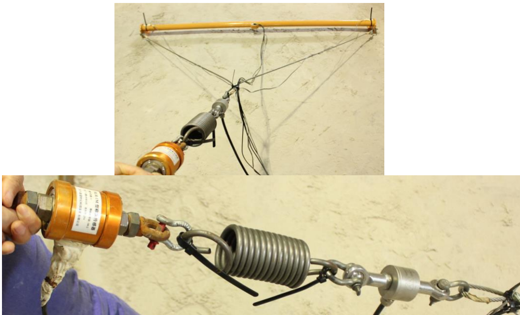
Figure 7-11 Load Cells in between the warp line
