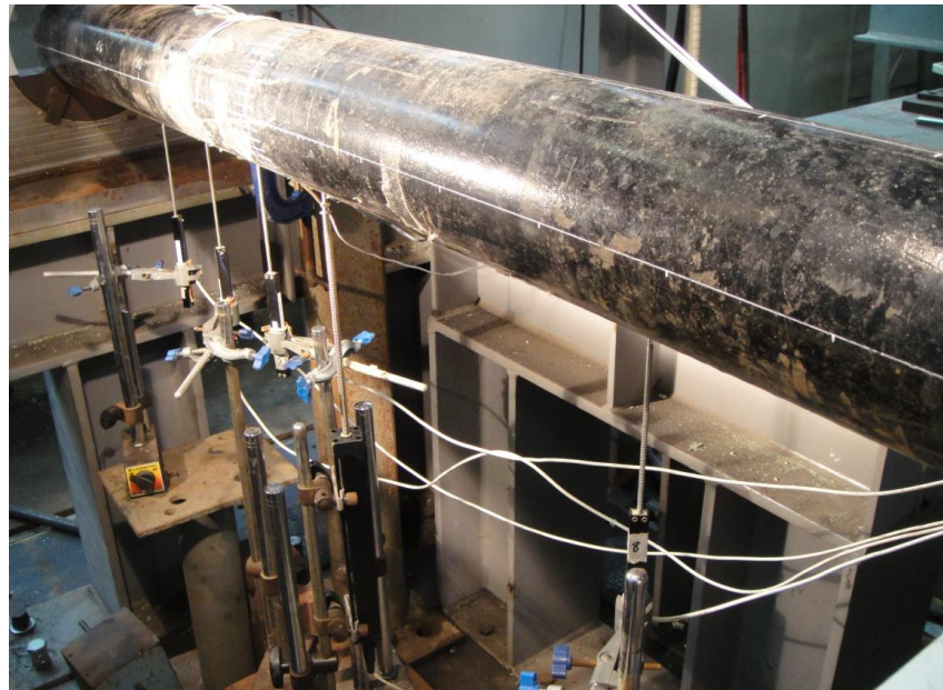
Figure 4-4 Strain gauge layout of single wall pipe or the outer pipe
