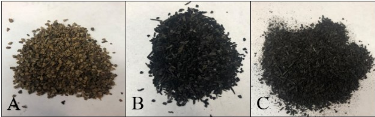
Figure 2.1 Sieved poultry litter (A), pine BC (B), and miscanthus BC (C) used in this experiment.
