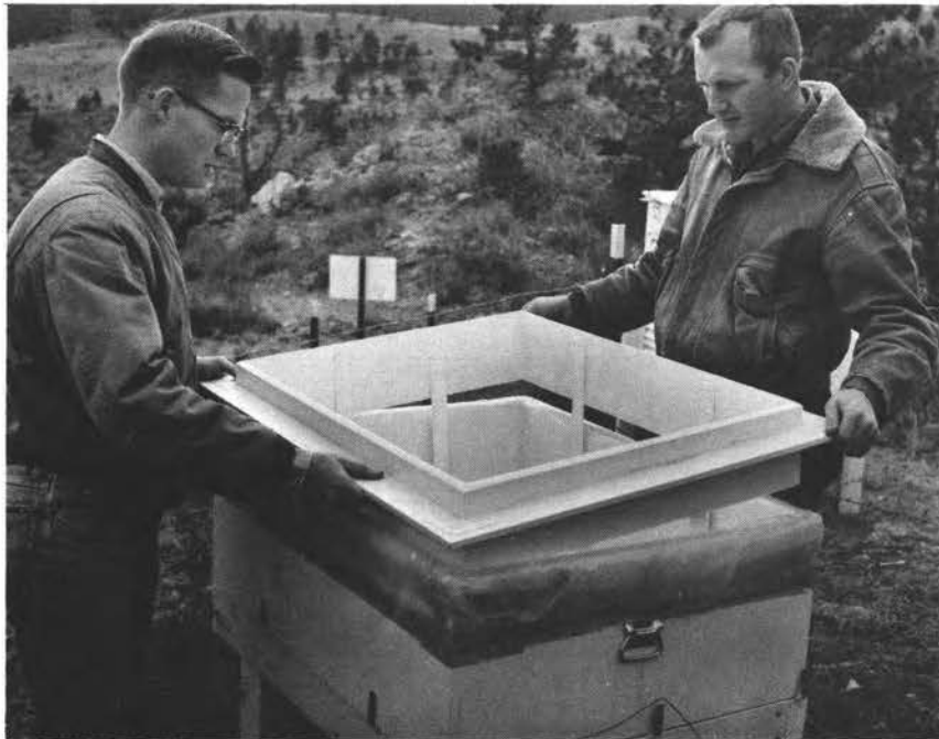
Fig. 12. The open collector at Kelly Flats which was used for rain, snow, and dust sampling.
