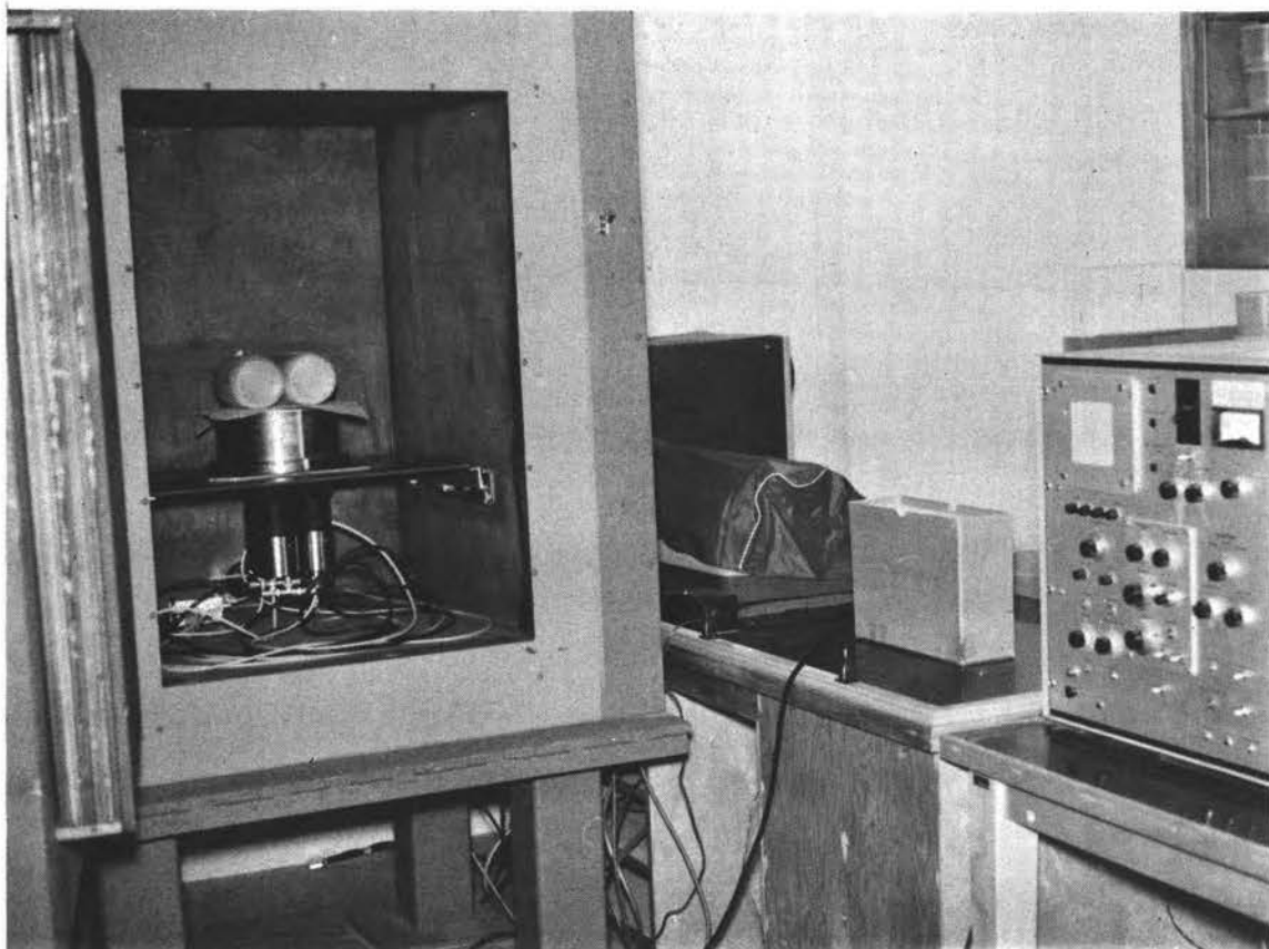
Fig. 17. Gamma spectrometric counting system used for various types of bulk samples.
