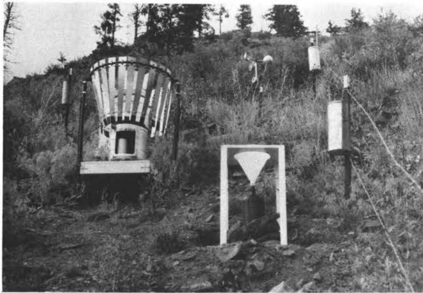
Fig. 11. Portion of weather installation showing polyethylene funnel used for rain sampling in foreground.
