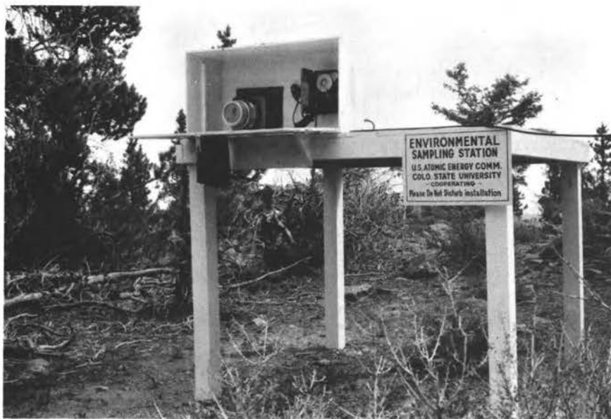
Fig. 10. Air sampling installation at Buckhorn Mountain.
