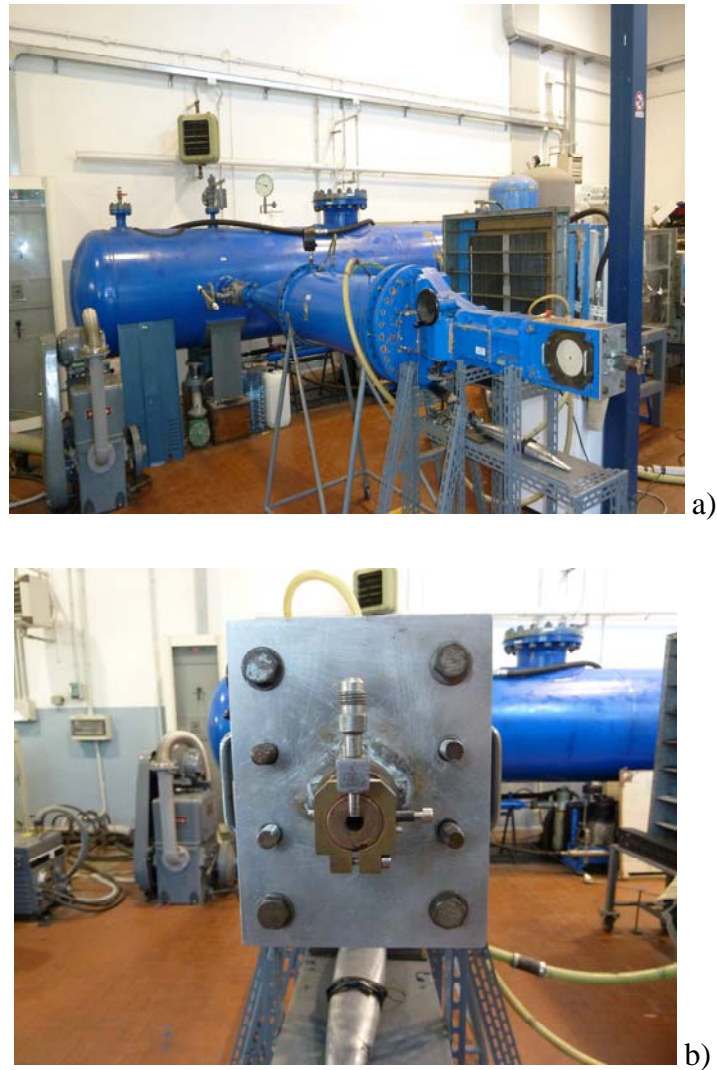
Figure 4: High Subsonic, Cold Flow Facility (a) global view (b) detail of injection zone.
