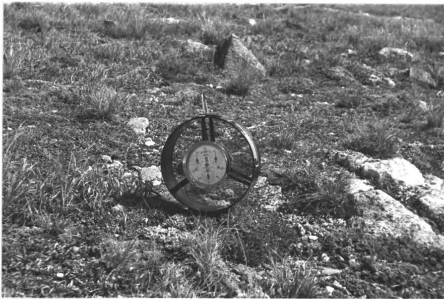
Figure 4.12. A portable wind meter, very sensitive at ground level used to measure the wind profile and speed.
