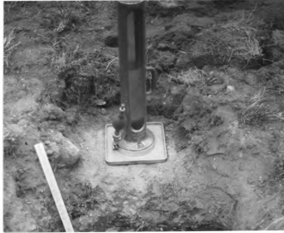
Figure 4.7. Volu-meter for measuring soil bulk density.
