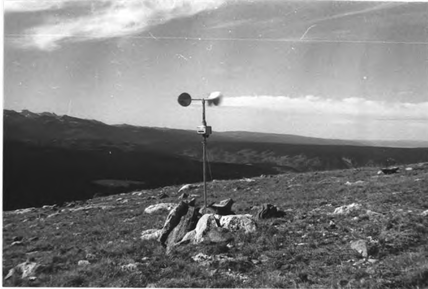
Figure 4.11. Totalizing wind anemometer used to measure the total passage of wind on Crown-Point study area.
