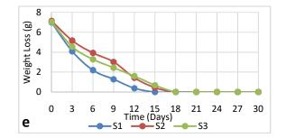
Figure 2. a–e: Line graph for 0.25, 0.50, 0.75 and 1.00 M H<sub>2</sub>SO<sub>4</sub>; and simulated acid rain (0.5 M HCl, HNO<sub>3</sub>, H<sub>2</sub>SO<sub>4</sub>).
