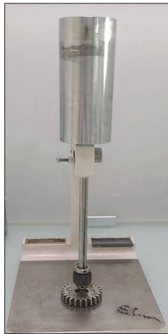
Figure 4: A 5 kg pressure was applied to standardize the step during the setting time of the luting agents
