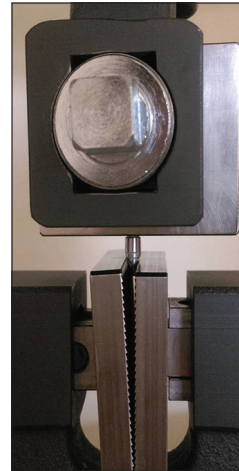
Figure 5: Customized holder that matches accurately with the specimen to keep them in place
