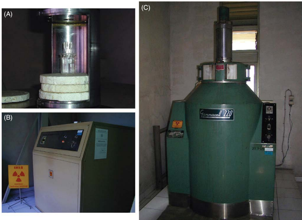
Fig. 12.1. Two gamma irradiators (A, B) Serial Type GC-4000 made in India and (C) model GC-220 made in Canada with an installed cobalt-60 source available at CIRA, BATAN for irradiating breeding materials in mutation breeding programmes.
