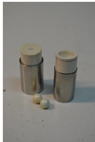
Figure 6. A homogenous sample was prepared by a mill (left image). Therefore, the samples were filled in the grinding beakers.
