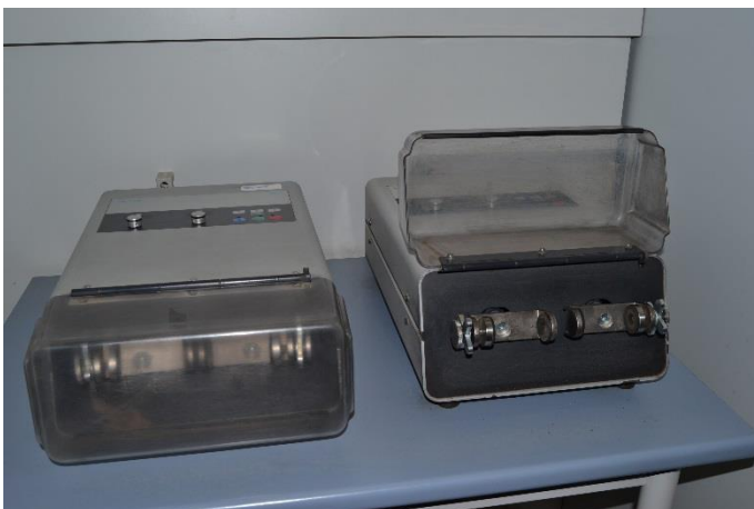
Figure 6. A homogenous sample was prepared by a mill (left image). Therefore, the samples were filled in the grinding beakers.
