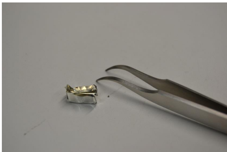
Figure 7. Tin boats, in which the samples are filled, have a size of 6 x 6 x 12 mm.
