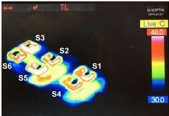
Fig. 19. Thermal image of the PUC converter by applying the traditional modulation method.
