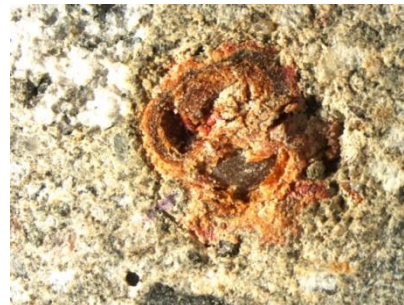
Fig. 5. -1-Middle-2: Leached out materials as observed in the sample
