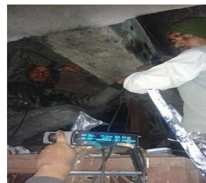
Fig. 3. UPV Measurement being recorded
