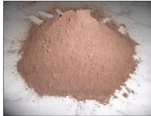
Fig 1. Slags of natural pozzolan before grinding. Fig 2. Powder of natural pozzolan after grinding < 80 \mu\text{m} .
