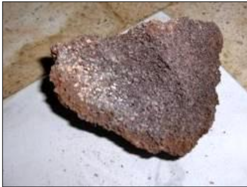
Fig 1. Slags of natural pozzolan before grinding. Fig 2. Powder of natural pozzolan after grinding < 80 \mu\text{m} .
