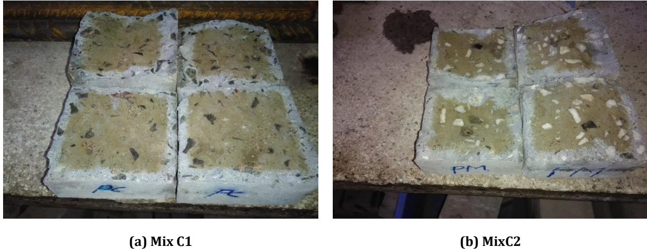
Fig 2. Images of chloride ion penetration of concrete.
