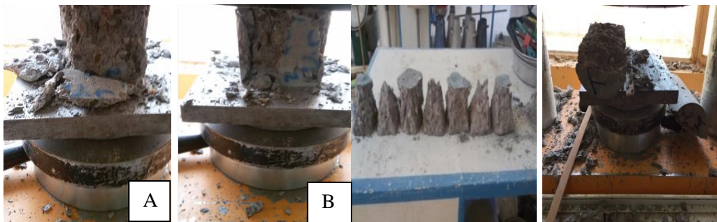
Figure 1: (a) & (b) Pattern of failure for N.C
