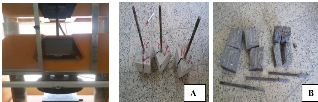
Figure 4: Pullout test machine
