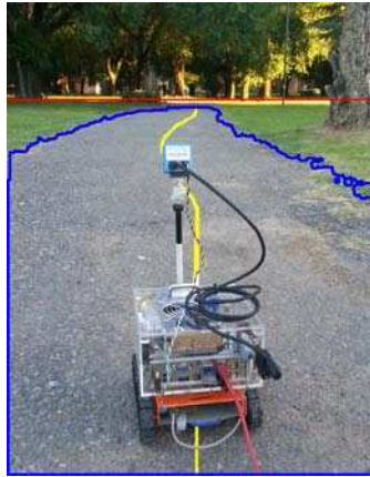
Figure 4.1: ExaBot robot performing autonomous navigation in an unknown outdoor environment. The horizon line (red) is detected as well as contour of navigable space (blue). Middle points of the road are computed (yellow) to guide the robot. To achieve real-time constraints imposed by robot motion, the image segmentation is implemented on a low-power on-board GPU (on top of the robot).
